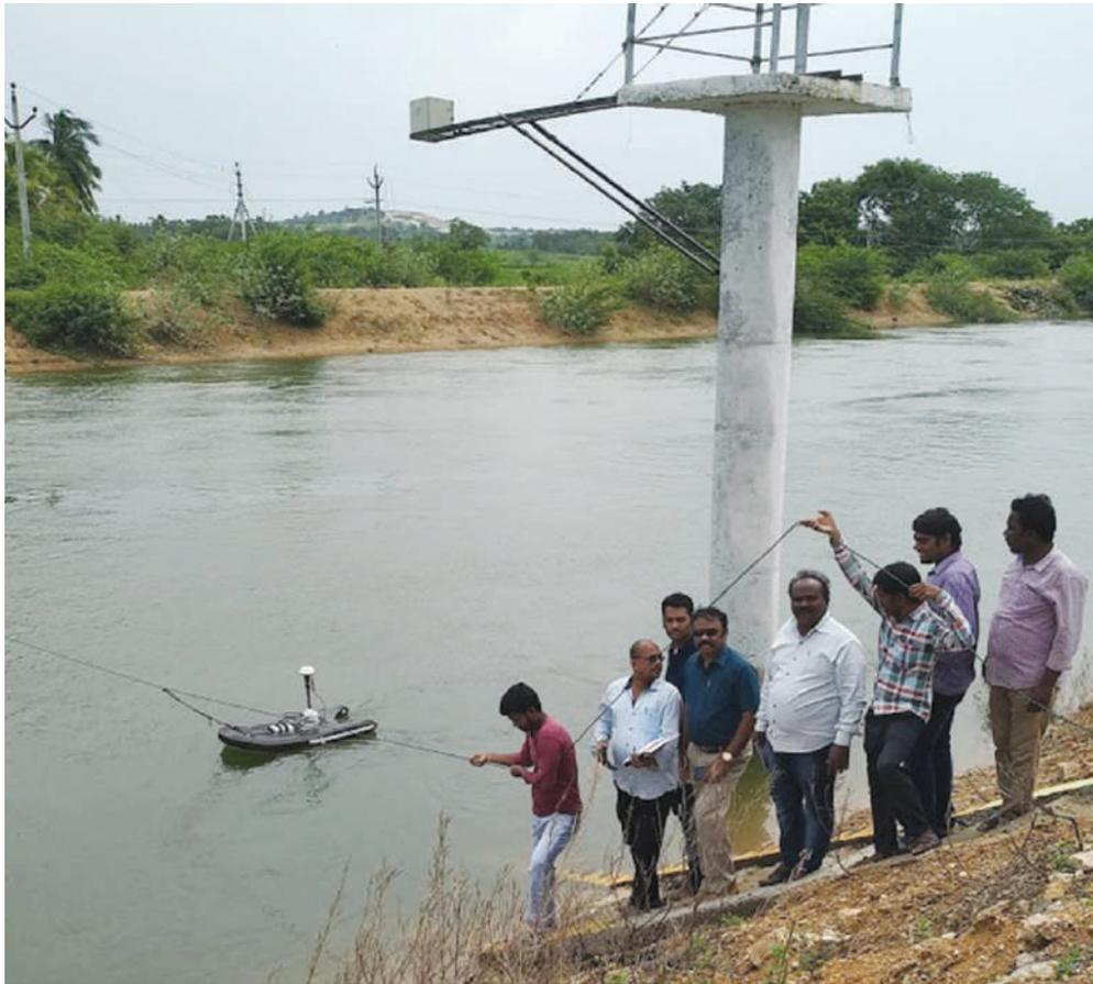
*Measuring discharge with ADCP at Paleru Off Take*
